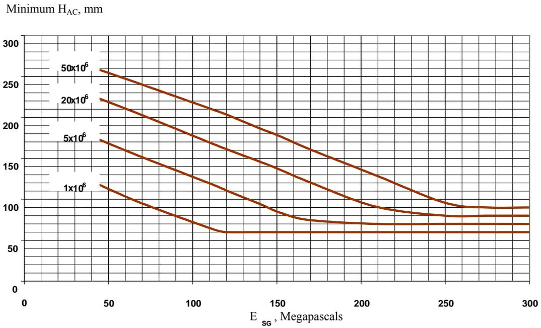
**FIGURE 3 Minimum Thickness of AC Layer for Flexible Pavements with  $H_P$  above 30 cm**
