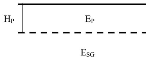
If the FWD loading plate geometry is applied onto the two-layer simplification of Figure 1, it is found that for a range of  $H_P$  thicknesses of 25 to 75 cm the ratio of  $E_P/E_{SG}$  is practically independent of  $H_P$ , and the following approximation can be adopted:
