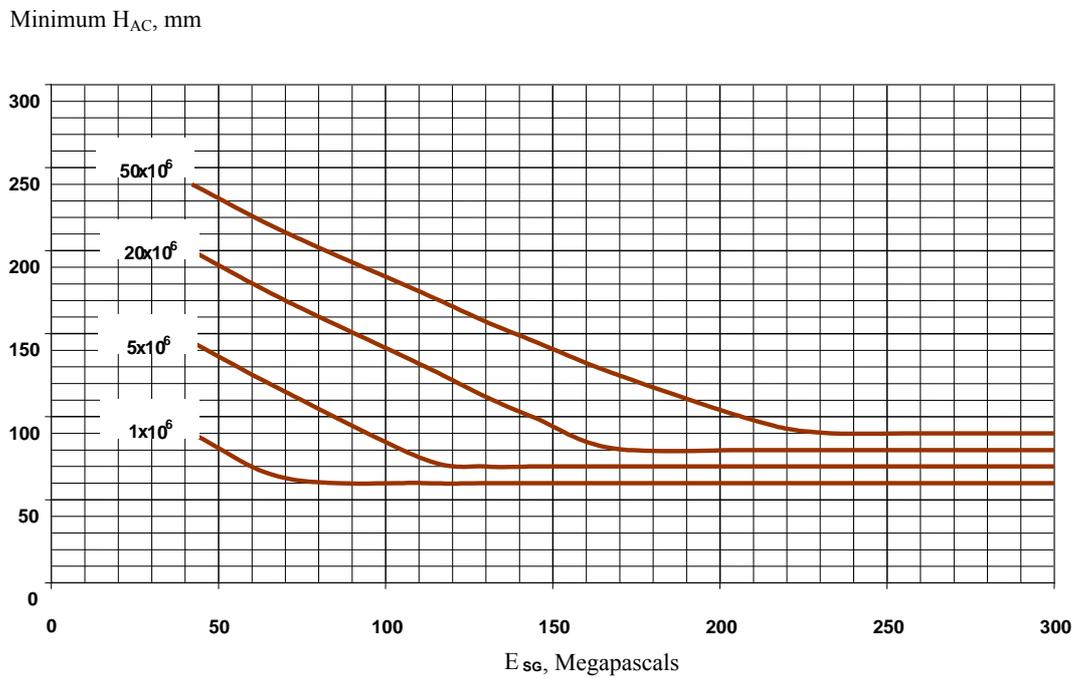
**Combining the minimum  $H_{AC}$  required with the existing AC layer**
